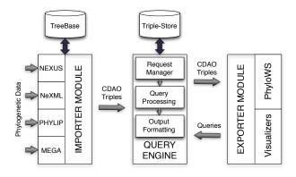
Figure 3: Overall structure of CDAOStore
